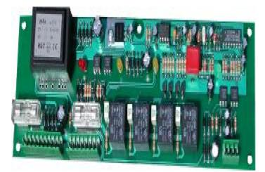
The Pcb generate the command sequence for: Power control. High frequency. Low pressure air valve High pressure air valve
