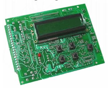
RE283 is a supervising board which gives reference welding voltages and wire speed, and performs welding tests, according to a user-defined program selected among 99.
