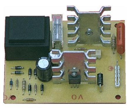
This board is intended to control a 24V-30W wire motor feeder and to switch directly (Max 220v-25A 15% duty-cycle).
