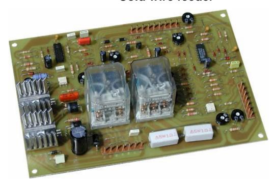
On the control card are present all the functions necessary to a cold wire feeder:
