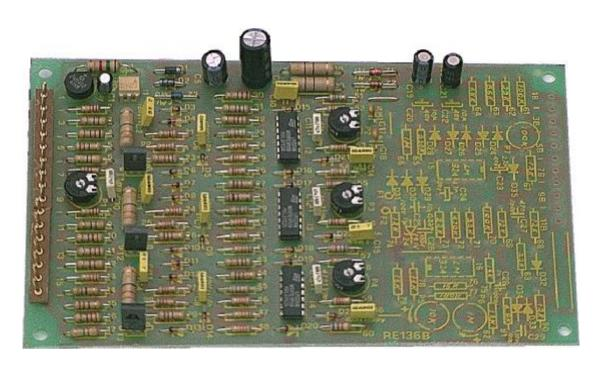
The card can be a erranged also for an half controlled 3 phase bridge in a electrade welding machine.
