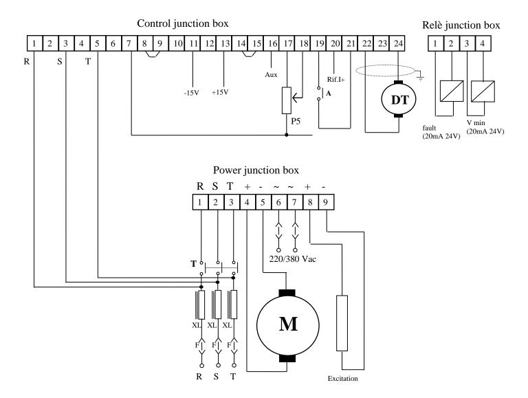
T: Power contactorsA: Drive enable switchXL: Line InductancesP1: Speed potentiometer
