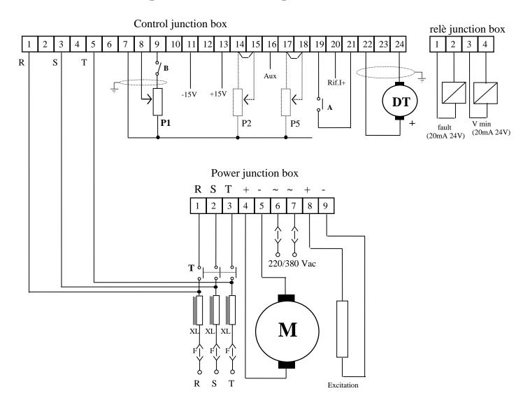
**T:** Power contactors **A:** Drive enable switch
